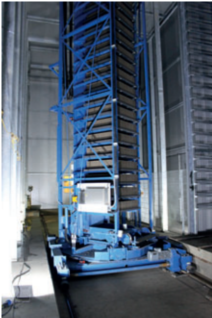
The platform of the finger car rotates by 180° during the journey.
