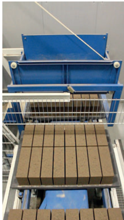
The production boards with the fresh concrete goods are transported into the elevator in the curing chamber by a conveyor belt.
