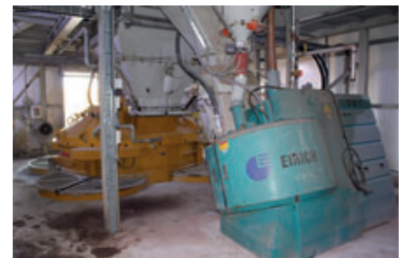
A Haarup mixer and an Eirich mixer supply the concrete block making machine with core and facing concrete.
