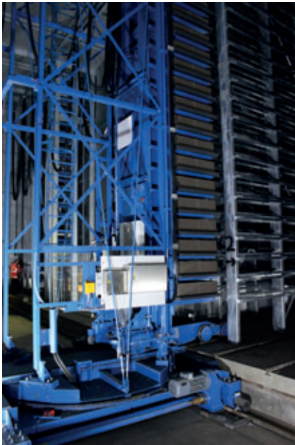
The finger car takes the cured products out of the rack chamber.
