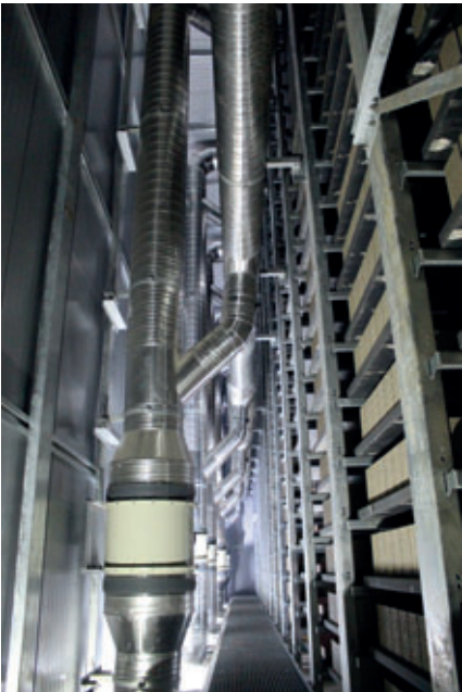
Circulation circuits of the ROTHO-ProCure system
