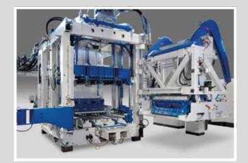
The complete face mix feed box of our KRS3 can be unlocked and swivelled sideways, in order to ensure an easy mould change and cleaning of the machine.
