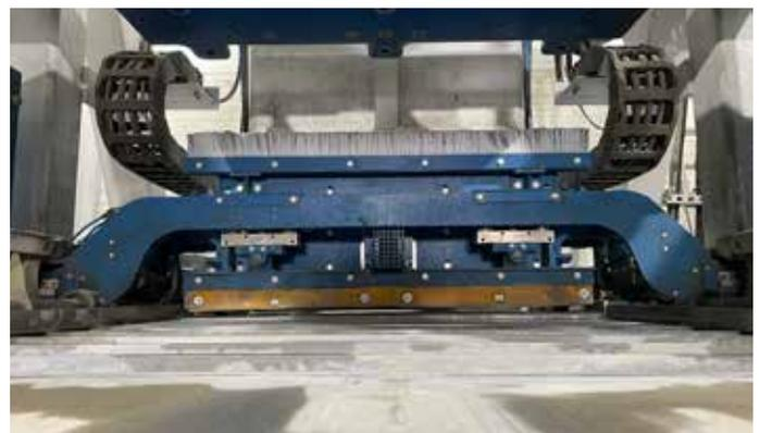
Finished green products are demoulded on a base board that is clamped on the mould or the vibrating frame before the tilting process. This largely eliminates product damage during the demoulding process. Another unique feature is the kinematics of the tilting movement by means of a frequency-controlled electric motor, which not only allows gentle movements but also works much more energy-efficiently than conventional hydraulic drives.
