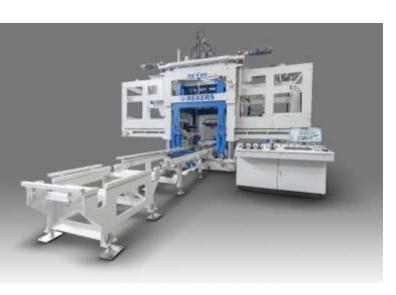
A special feature of this machine is that, unlike conventional machines, no lifting of the face mix section (approx. 7 tonnes) is required. This technological innovation leads to a considerable increase in efficiency. The RS4 is up to 50% more energy efficient than comparable hydraulically operated machines, which not only leads to an improved environmental balance, but also to cost savings.
