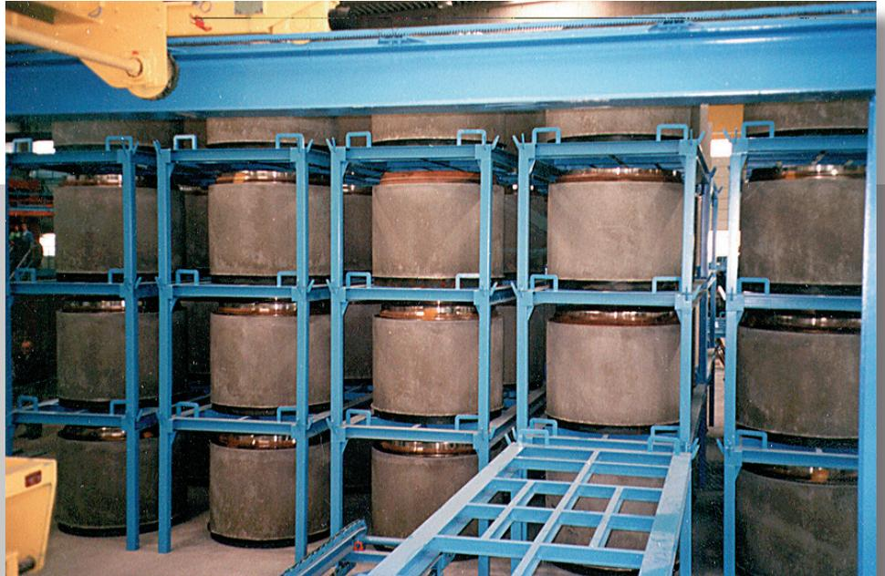
*Product in self-stacking racks for efficient curing within a minimum floor area. Product size from 800 - 1500 mm diameter and height to 2000 mm.*
